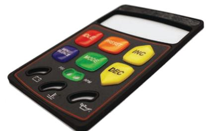
If the device has a thicker or sculpted exterior package, the dome can be activated with an actuator.
