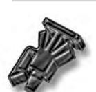
Heavy duty nylon 6/6 support snaps into P.C. board from bottom. Locking arm clips to the side of the P.C. board making for easy removal and replacement of P.C. boards. Support does not rotate in chassis or positioning holes. Board clearance may vary depending on chassis thickness. Parts are molded in black nylon.
