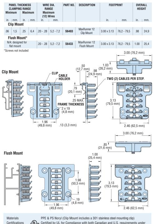
$_{c}(\Psi_{L})_{us}$  Certified by UL for Compliance with both Canadian and U.S. requirements under File E54523 Flammability Rating 94V-0
