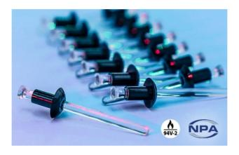
These rivets have a nylon rivet body and a clear polycarbonate mandrel, they are set in the same manner as metal pop rivets with a standard installation tool.
